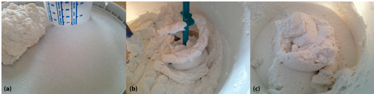
Figure 1. Various steps of the mixing: (a) original components; (b) mixing phase; (c) final composition of the plaster.
