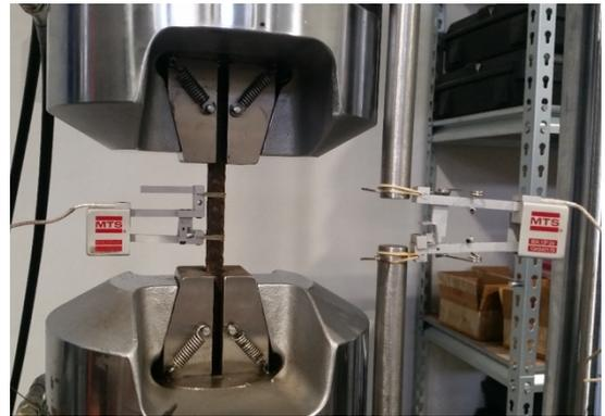
Figure 6 Test set-up employed in order to perform the low-cycle fatigue tests.
