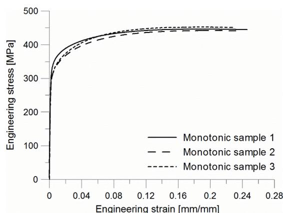
Figure 4 Stress–strain curves of the benchmark samples.
