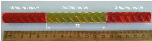
Figure 5 Reinforcing bar specimen used for the experimental testing. Gripping and testing region are specified (dimensions are in mm).
