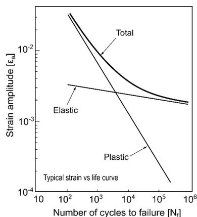
Figure 3 Typical strain versus life curve.
