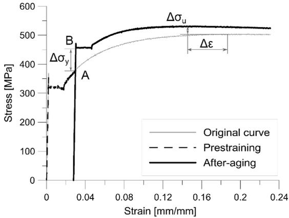
Figure 1 Stress–strain curve of NZ-manufactured Grade 300E subjected to strain ageing
