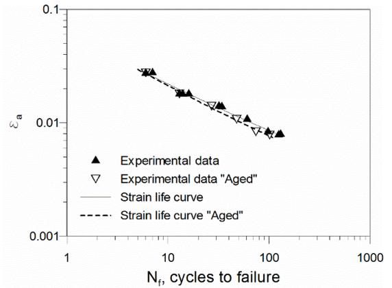
Figure 8 Comparison between unaged and aged samples (66% precycled). Coffin–Manson model using total strain.
