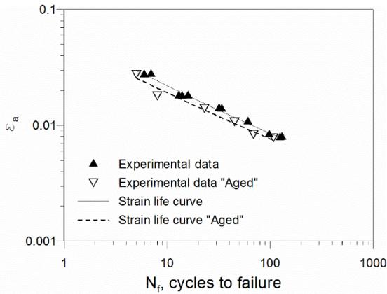
Figure 7 Comparison between unaged and aged samples (33% precycled). Coffin–Manson model using total strain.
