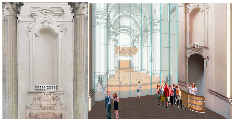
Fig. 7. Design view of the atrium. On the right side, multidirectional nozzles are visible, installed in the recess with a plasterboard wall to hide the presence of the air channel.
