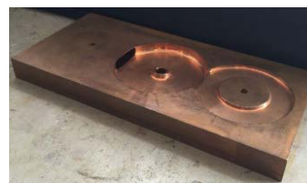
Fig. 3. OHFC 99.99% copper back-to-back cell after the brazing process
