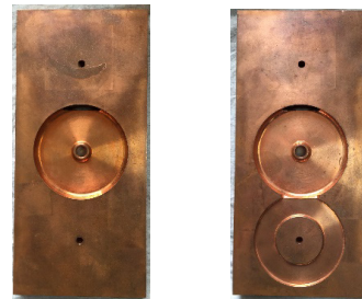
Fig. 2. . OHFC 99.99% copper half-cell plates showing a coupling half-cell (left) and an accelerating half-cell (right).
