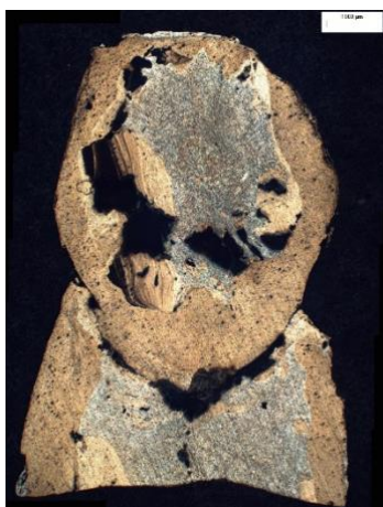
Fig. 7: metallography of the vertical section of the extruded wire.
