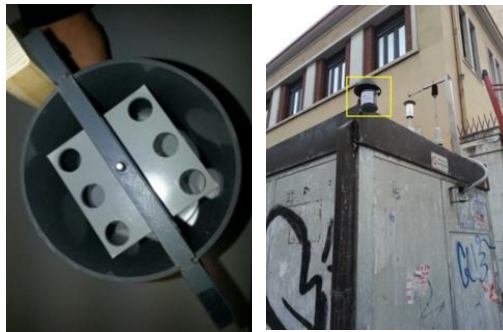
Fig. 4. A passive sampler holder in situ in Viale V. Veneto (note the yellow square).
