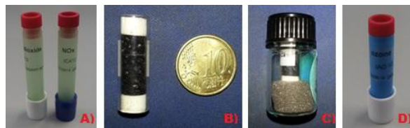
Fig. 5. Passive samplers: A) for nitrogen dioxide and nitrogen oxide, B) and C) for BTX, D) for ozone.
