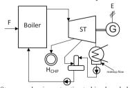
Fig. 2. Steam condensing extraction turbine-based plant
