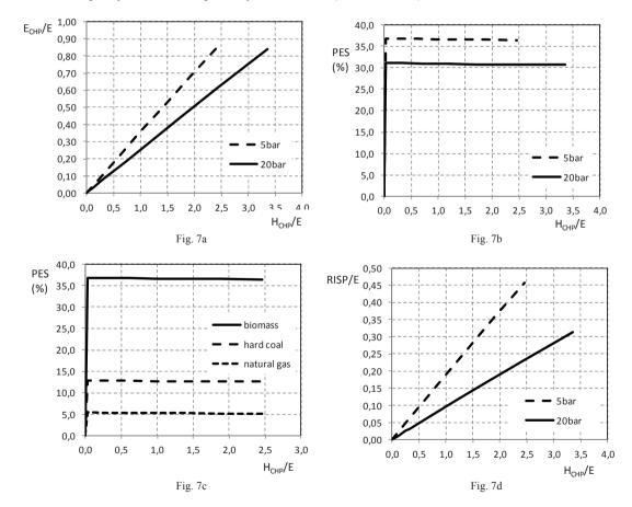
Fig. 7a shows the trend of the ratio of the CHP electricity to the total electricity: the heat demand at higher quality, that is at a higher temperature, penalizes this parameter because an higher extraction pressure involves an increases of the value of  $\beta$  and thus a decrease of the power to heat ratio ( $C_{eff}$ ) while the efficiency of non-combined electrical energy generation remains approximately constant. In this analysis the main average results are:
