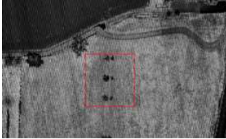
Figure 1a. Example of an area with homogeneous ground points intensity and darker vegetation points.
