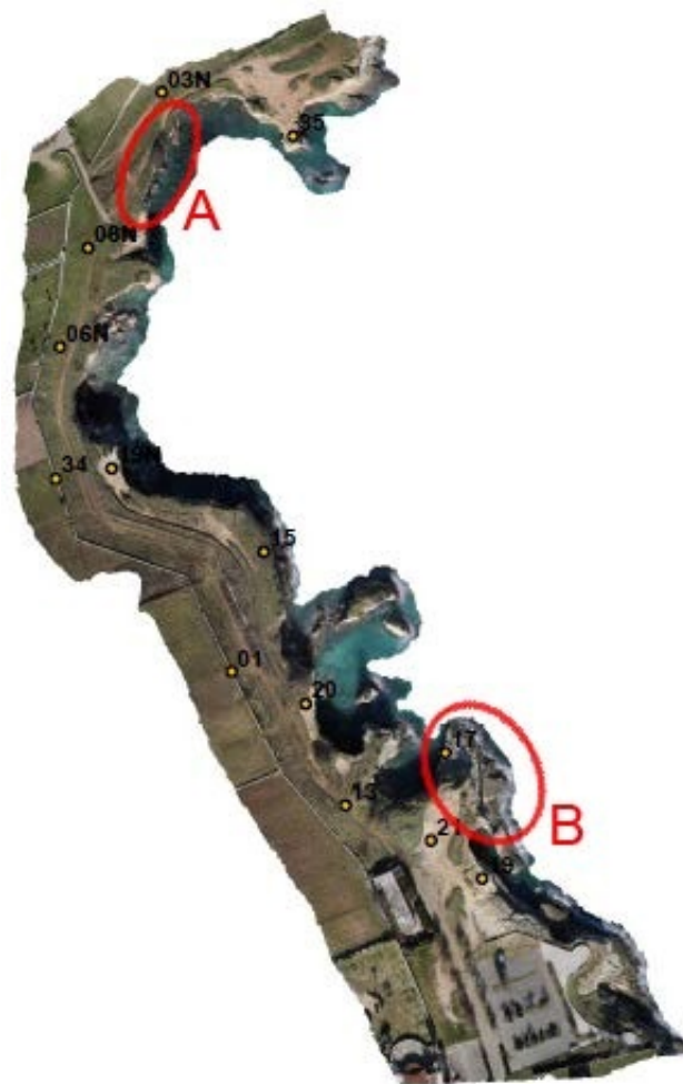
Figure 3: The location of Ground Control Point (GCP)
