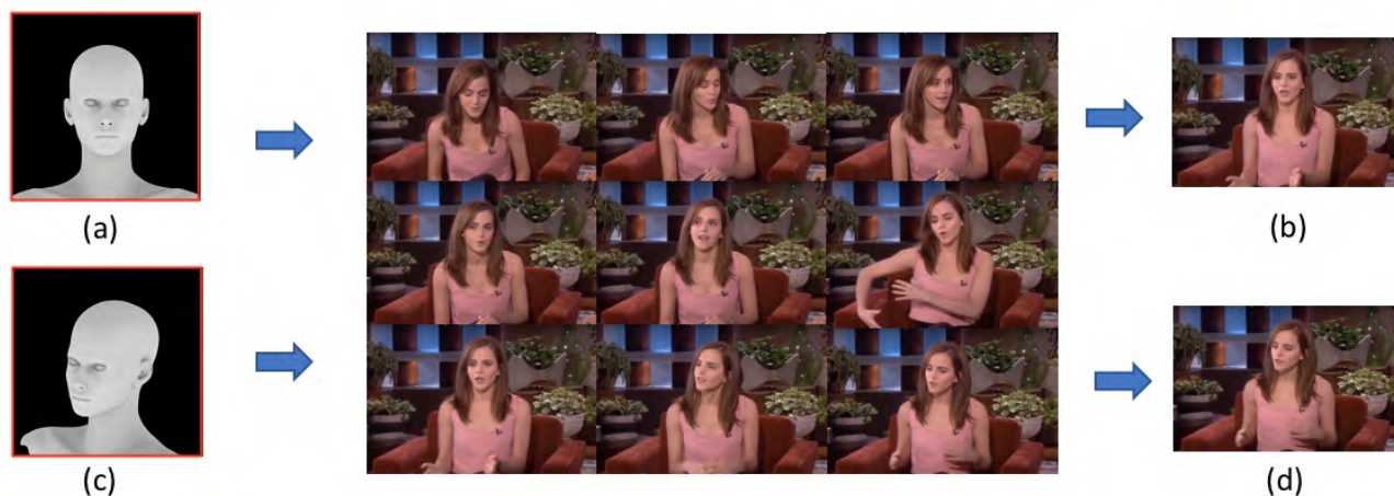
FIGURE 11. Search for the desired pose in a sequence of frames extracted from a video interview (a) Search for an image that matches the frontal pose of the synthetic model with angles: P +00, Y +00, R +00 (b) Front-most frame in the sequence (c) Search for an image that matches the synthetic model with angles: P +10, Y +30, R +05 (d) Frame more similar to the required pose.
