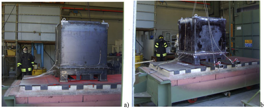
Fig. 4. Positioning of the mock-up on the slide of the oven before (a) and after fire test (b).
