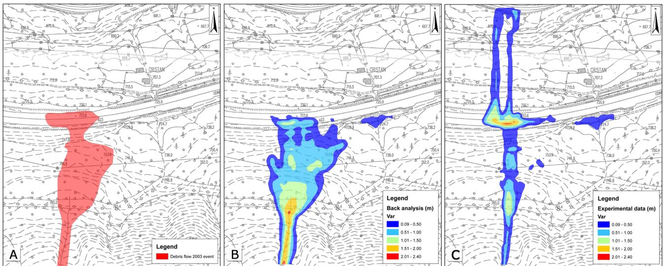
**Fig. 7.** (A) Inundated area bounded just after the 2003 alluvial event; (B) back-analysis simulation: inundated area and debris thickness with rheological parameters from Aspen Watershed model; (C) scenario of debris-flow event simulated with rheological parameters obtained through experimental data.
