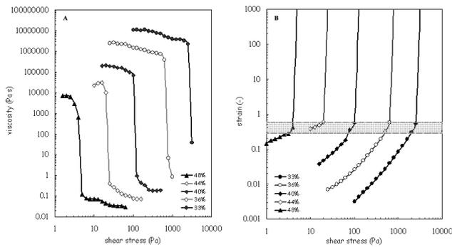
**Fig. 4.** (A) Plastic behaviour shown by the investigated samples; (B) strain range (gray stripe) representing data from small but continuous deformation to appreciable flow conditions.
