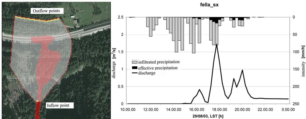
**Fig. 6.** (A) In light grey: computational domain area. Inflow point at the top of the fan (yellow point), outflow points downstream (yellow line). (B) Complete hydrograph: only a part of it has been used as input parameter for the simulation, 16h00–18h50
