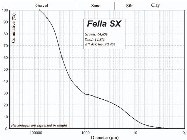
**Fig. 3.** Grain-size cumulative distribution for the sample collected at the Fella sx watershead.
