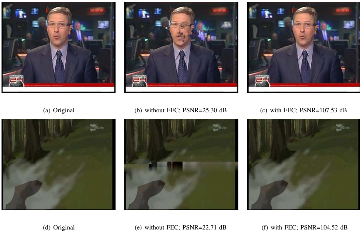
Figure 3 Comparison of visual effects on decoded frames for the videos 'News' and 'Cartoon' at 2 Mbps with and without FEC technique. The overhead is equal to 20%, and PLR is equal to 3%.
