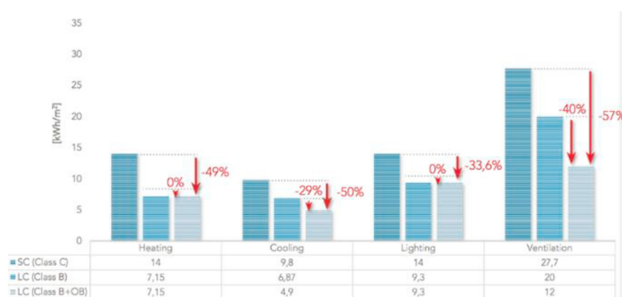
Fig. 4. Energy performances of SC and LC with BAC and window opening preferences.
