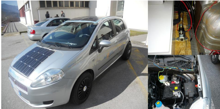
Fig. 3. HSK installed on a FIAT Grande Punto and some wiring details.
