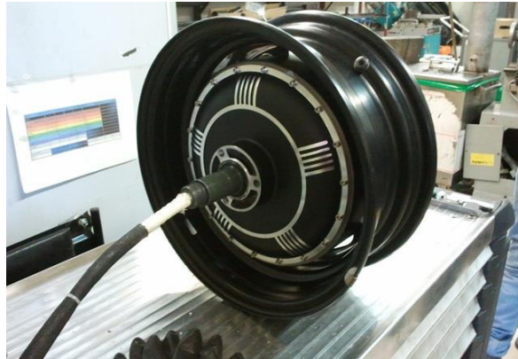
Fig. 5. Kelly Controls in-wheel motor 96V 7 kW.
