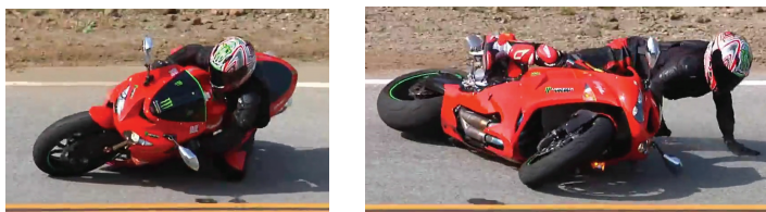
Fig. 5. (a) the initial stage of lowside; (b) the lateral fall. (Source: youtube.com)
