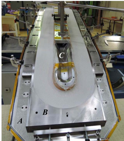
Fig. 5. Winding setup after completion of layer 4, showing (A) the winding table, (B) one horseshoe, and (C) the central post.
