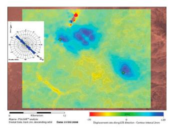
Figure 3:Raster image and contour lines of maximum displacements measured along satellite LOS compared to strike of the main conductive fracture system.
