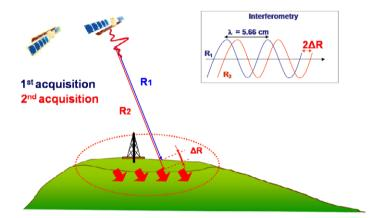
Figure 1: A schematic showing the relationship between ground displacement and signal phase shift. The numeric value of the wavelength  $\lambda$  is that used by the ERS satellite operated by the European Space Agency (ESA).
