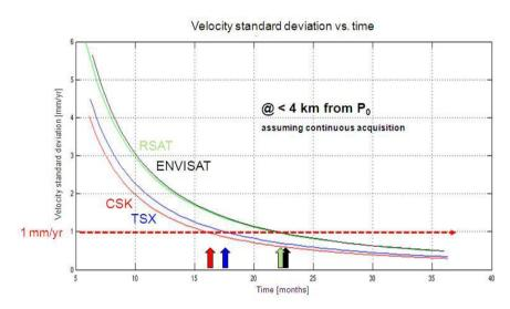
Figure 2: Precision of multi-interferogram InSAR measurements as a factor of satellite platform used and the number of months of data acquisition.
