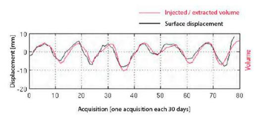
Figure 5:Comparison between vertical surface displacement measured with satellite data processing and injected/extracted gas volumes
