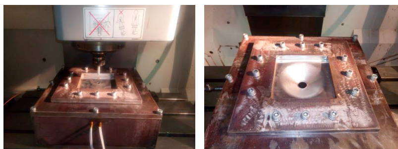
Fig. 1. ISF equipment and parts at the end of the process.
