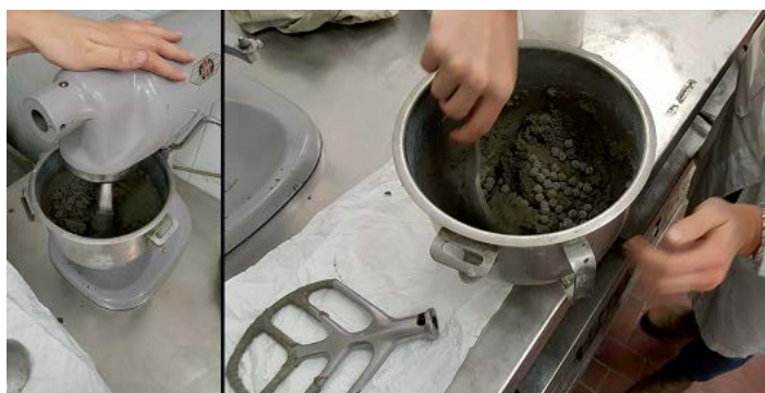
Fig.5. Mixing procedure of self-healing mortar.
