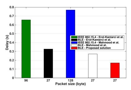
Figure 12. End-to-end delay of the WNs.
