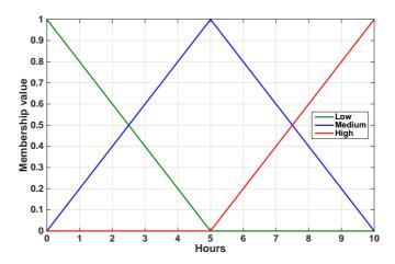
**Figure 6.** Triangular membership functions for the scheduled time of the input and output parameters for the FLC.
