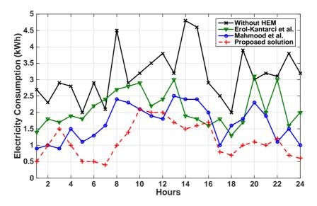
Figure 7. Peak load reduction comparison.
