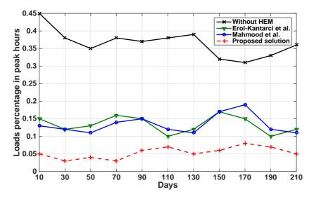
Figure 8. Load of the appliances ratio during peak hours.
