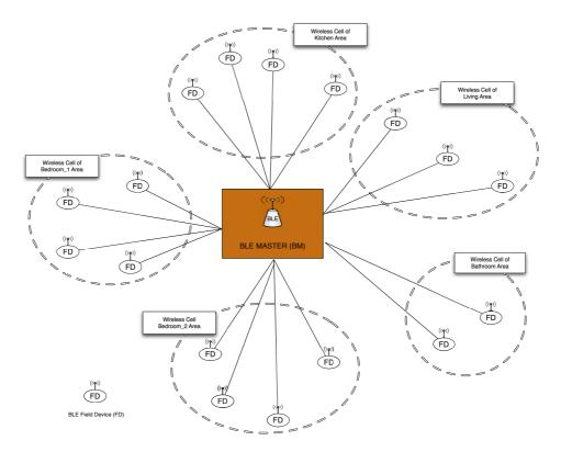
Figure 2. The proposed BLE-based wireless network topology.
