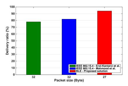
Figure 11. Delivery ratio of the wireless networks (WNs).
