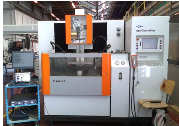
Fig. 1. The sensor monitoring system mounted on the wire EDM machine
