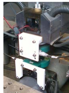
Fig. 2. Detail of the current and voltage sensors.
