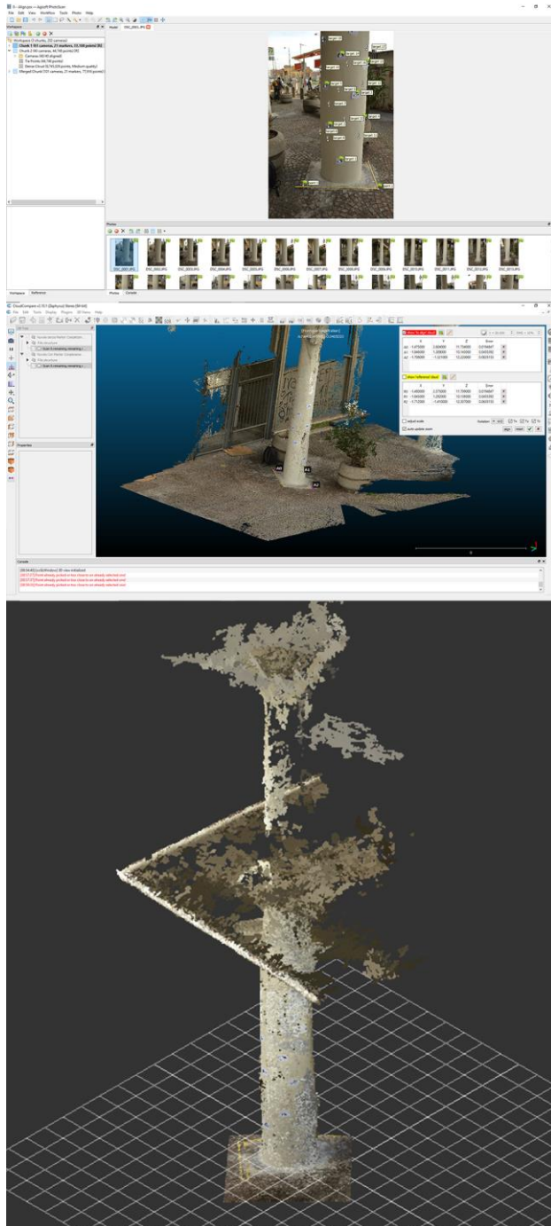
Figure 4. Creating the column point cloud. On the top, reconstruction of the point cloud through digital photogrammetry. On the centre, cleaning phase. On the bottom, final phase and results.
