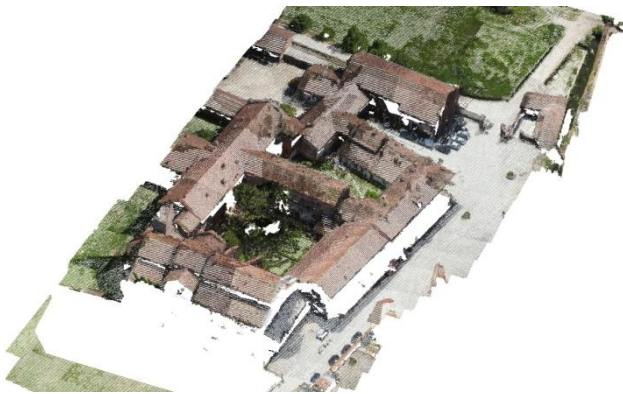
Figure 15. Point cloud extracted using Photoscan software
