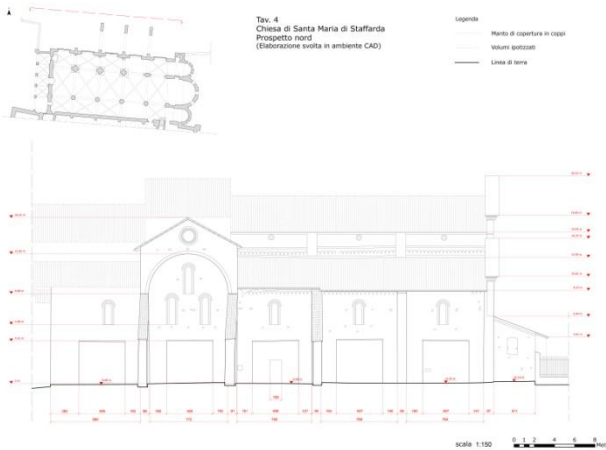
Figure 6. North front processed from laser scanner data
