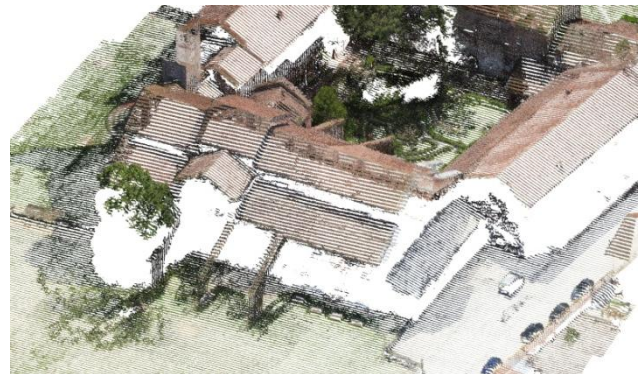
Figure 27. Point cloud extracted from Photoscan. This zoom on the Church allows to notice the noise affecting the cloud.
