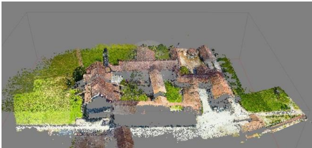
Figure 10. Calculated Tie Points in Photoscan
