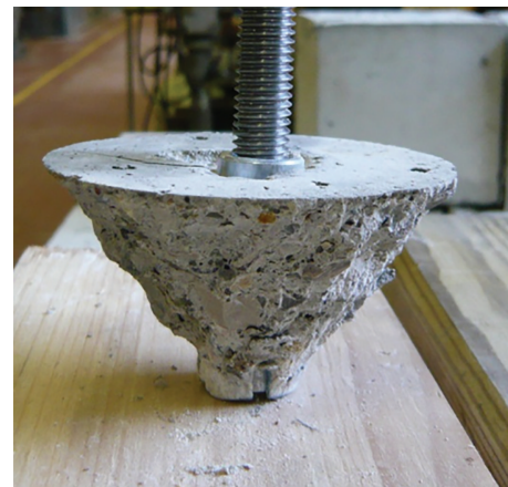
FIGURE 7: Extracted cone by the B15G sleeve.
