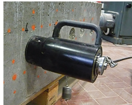
FIGURE 9: Pull-out of unloaded concrete.
