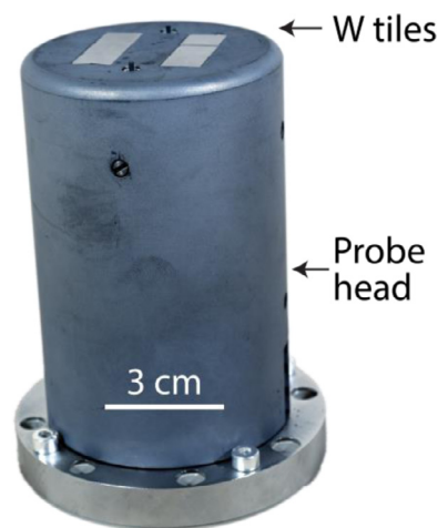
Fig. 2. Samples installed in the manipulator before exposure to He-ICWC.
