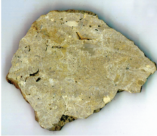
FIGURE 8: Micritic limestones with extensive vuggy and spongy fabric; maximum dimension of cavities is 1 cm, Sasso Streghe (number 10 of Figure 1).
