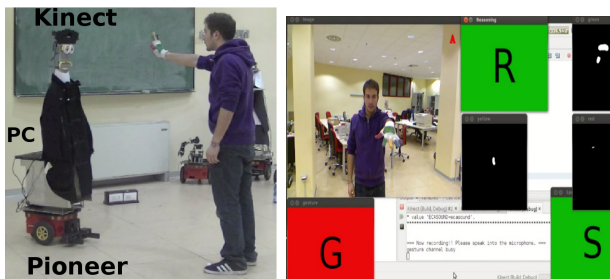
Fig. 3. Multimodal interaction with a mobile platform: a picture of an interaction and a screen-shot from the developed multimodal tool.
