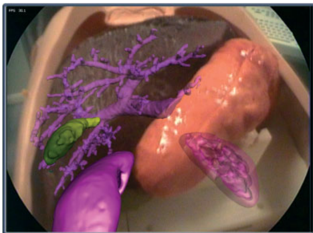
Figure 11. Screenshots of a mixed reality environment: portal system, gallbladder and kidneys are virtually mixed to the actual video streaming coming from an endoscope
