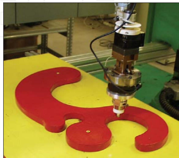
Fig. 13. The SCARA robot during the contour tracking of a complex shape
