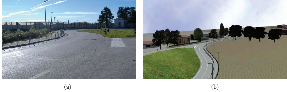
FIGURE 5: Real environment (westbound picture) and virtual environment (eastbound drawing): representation of the S-shape curve and the intersection.
