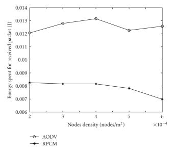
FIGURE 8: Performance of AODV and RPCM in terms of energy spent for received packet, when f = 6.
