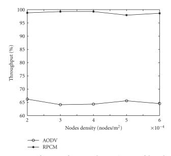
FIGURE 6: Performance of AODV and RPCM in terms of throughput, when f = 6.
