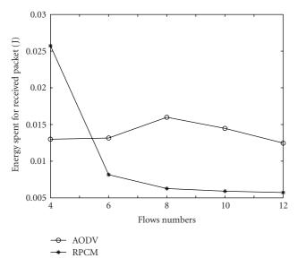
FIGURE 11: Performance of AODV and RPCM in terms of energy spent for received packet, when  $\rho = 4$  (nodes/m<sup>2</sup>).
