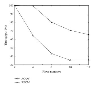
FIGURE 9: Performance of AODV and RPCM in terms of throughput, when  $\rho = 4 \text{ (nodes/m}^2)$ .
