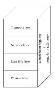
FIGURE 1: Protocols' stack integrated with mobility management.
