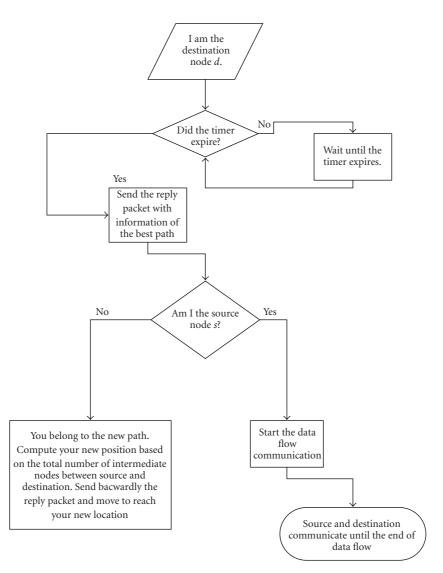
FIGURE 3: Reply phase of RPCM.
