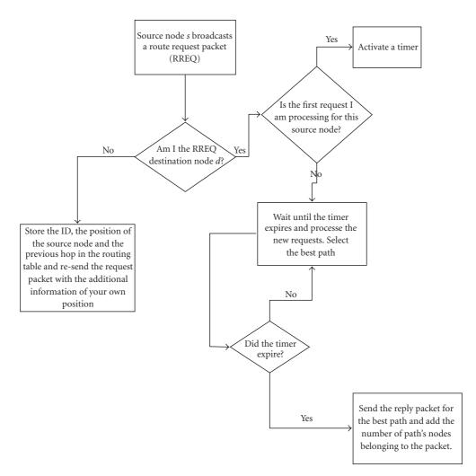
FIGURE 2: Routing Request phase of RPCM.
