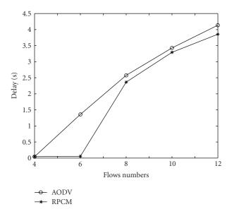
FIGURE 10: Performance of AODV and RPCM in terms of delay, when  $\rho = 4 \text{ (nodes/m}^2)$ .
