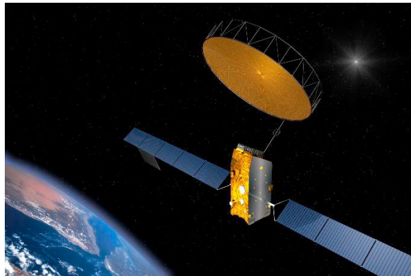
Fig. 1. AstroMesh® Reflector ( https://news.northropgrumman.com ).
