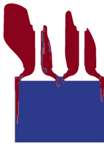
Fig. 3: Mean M parameter close to valve ports for valve lift 5 mm. In red the regions with M > 0.2
