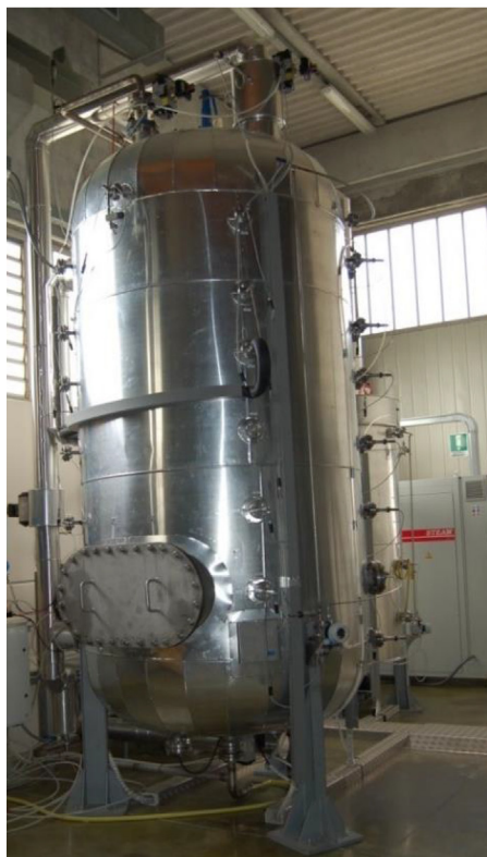
Fig. 4. (a) The thermally insulated condensation tank and (b) the subdivision of the inner volume in layer (with sensors identification and positions) (Huang et al., 2015).
