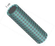
Fig. 5: CAD model of the PDMS substrate with the deposited periodic pattern: cylindrical surface
