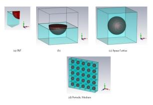
Fig. 4: Schematic representation of periodic medium made of spherical inclusions in a host medium
