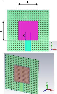
Fig. 9: Overall view of the MPA (top) and MTM substrate (bottom)
