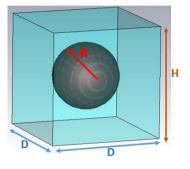
Fig. 7: Unit Cell of the MTM
