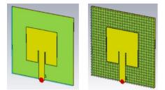
Fig. 1: Schematic representation of MPA with homogeneous substrate (left) and MPA with MTM substrate (right)
