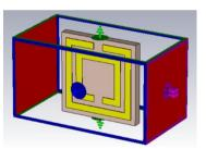
Fig. 8: CAD model for the Nicolson Ross Weir Method setup used to find the determination of the S-parameters
