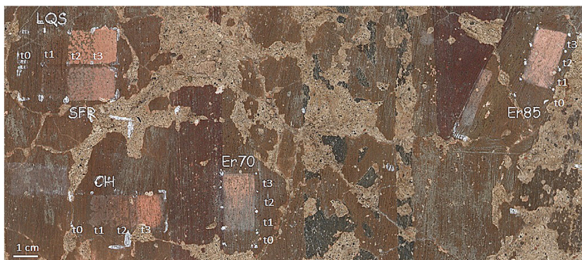
Fig. 1. Output of cleaning methods (labels described in Table 1) applied on the Sansepolcro fresco (t0 before cleaning and t1–t3 progressive cleaning steps).
