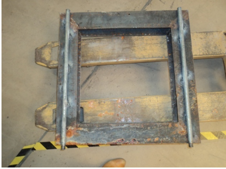
Figure 3: Bearing support frame structure
