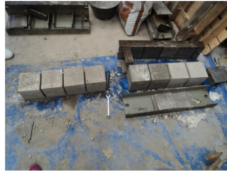
Figure 2: Concrete samples for compressive test
