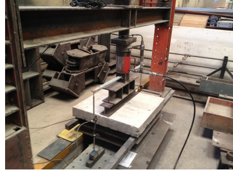
Figure 4: Testing configuration for reference sample
