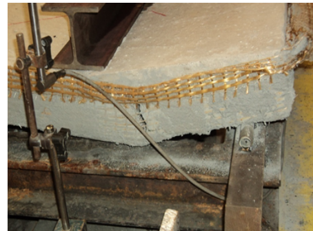
Figure 12: Collapse mode for the strengthened sample
