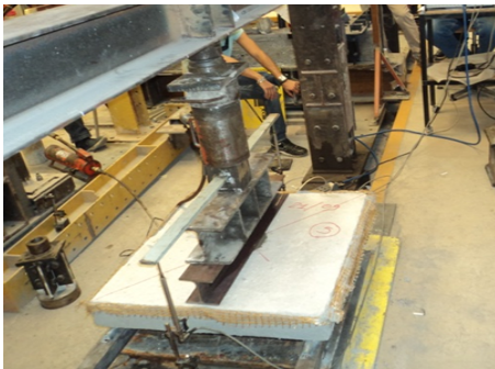
Figure 11: Testing configuration for strengthened sample
