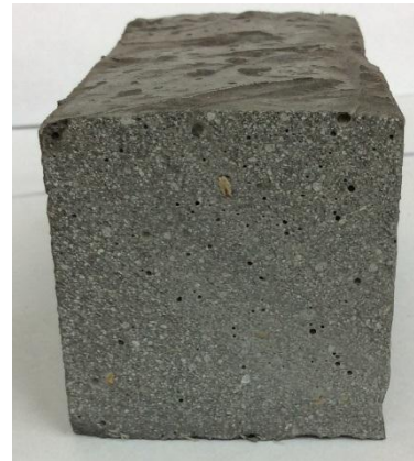
Figure 4. Sample with 1 % of green tow flax fibres, made by traditional casted method.
