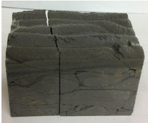
Figure 5. Plain sample made by injected process (simulation for 3D printing process).
