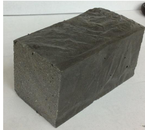
Figure 6. Sample made by traditional casted technology.
