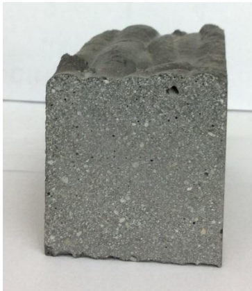
Figure 3. Plain sample (without fibres) made by injection method.
