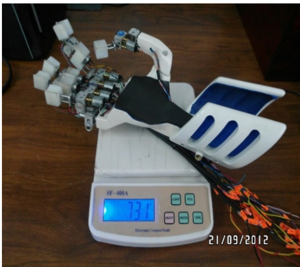
Figure 8. Rear part and weight of the exoskeleton
