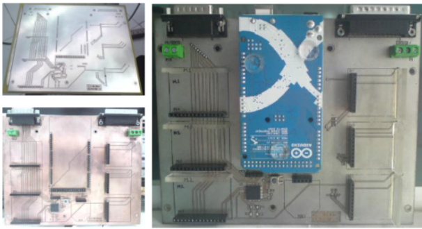
Figure 10. Motherboard PCB design
