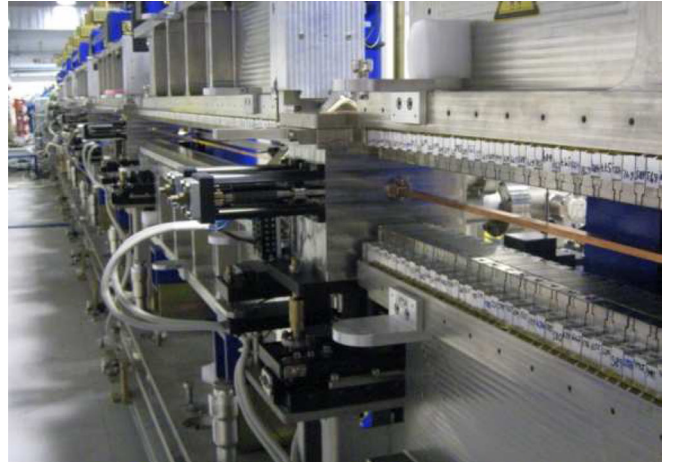
FIG. 3. SPARC undulator consisting of six sections made by 75 periods of 2.8 cm each (77 periods including two termination periods), with gaps variable in the range from 25 to 8.4 mm (limited by the vacuum chamber) corresponding to a maximum undulator parameter K_u \sim 2.2 (see definition below) at the minimum gap.
