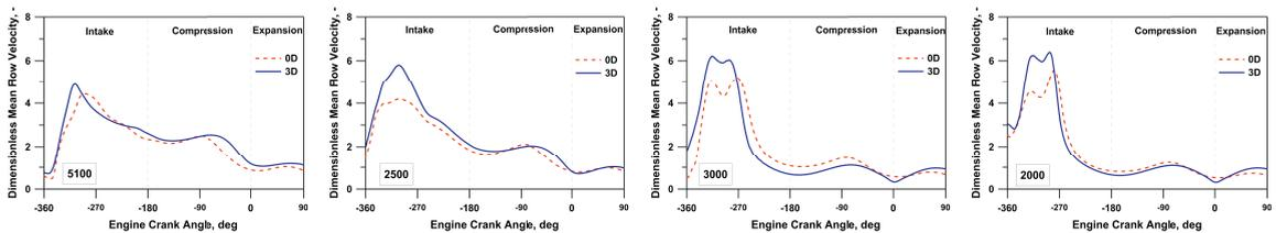
Figure 7. Dimensionless mean flow velocity 0D/3D comparison
