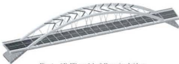
Fig. 4 3D FE model of Canonica bridge
