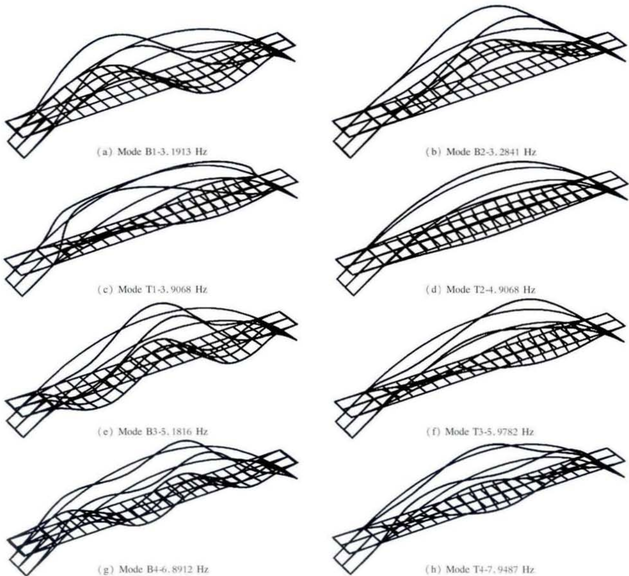
Fig. 13 Mode shapes of updated FE model
