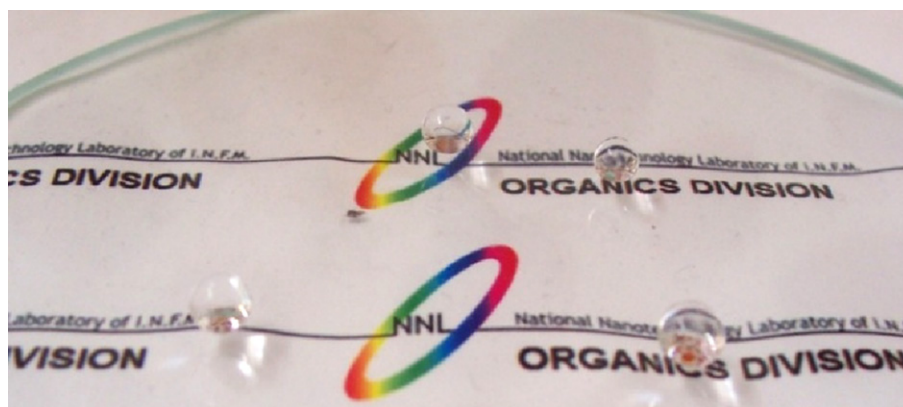
Fig. 9. Superhydrophobicity of transparent coatings on glass [58].
