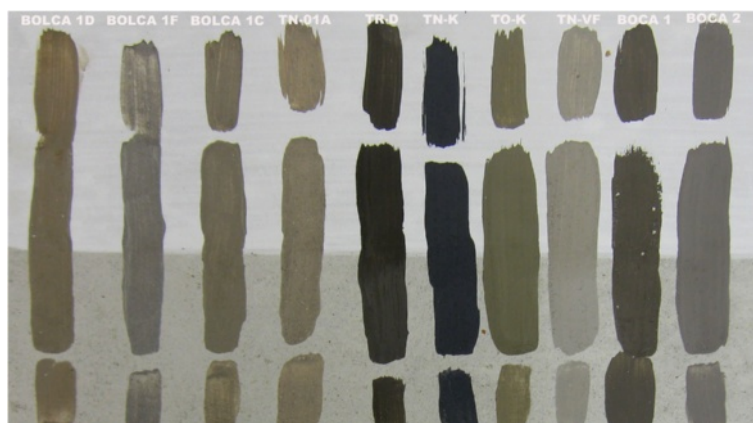
Figure 12 Replica of lime-based painting techniques using different black pigments: the picture shows the different colour of the black pigments both raw and manufactured after application with lime depending by the chemical composition and the particle size. The ground of the plaster (upper part) was smoothed with limewash whilst the surface of the lower part was left irregular. Pigments identification as follows, from left to right: Bol1d (5YR 5/6), Bol1f (5YR 7/2), Bol1c (10R 7/4), TN01a (10R 7/4), TR-D (5YR 2/1), TN-K (5YR 2/1), TO-K (5YR 3/4), TN-VF (5YR 5/2), Boc1 (5YR 5/2), Boc2 (5YR 2/2).
