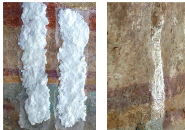
Fig. 7 On the left, application of EAPC and XYL systems for test experiments on the paintings “de los discos solares” in Mayapan, Mexico. On the right, the same area is observed after the removal of polymer coating. Under glazing light, the disappearance after treatment of the shining effect due to the coating can be appreciated. The presence of the polymer is evident in narrow strip that was left untreated.
