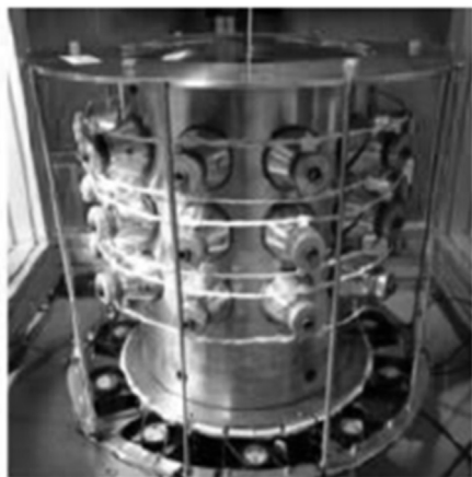
Fig. 4. NPL frequency driven reference ultrasonic vessel (25 l; 25 kHz) [17].
