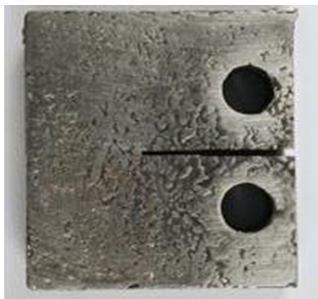
Figure 1: Macrograph showing the CT specimen.
