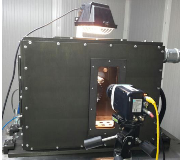
Fig. 2. High speed camera and illuminator setup.
