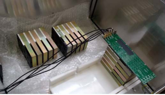
Fig. 3. Prototype during installation: the three longitudinal blocks are visible together with the PCB hosting the SiPMs.
